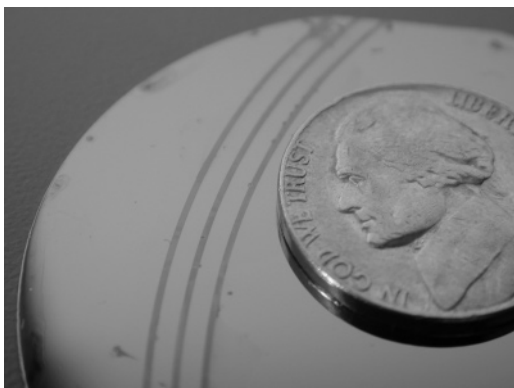
Figure 3. Image of a small silicon wafer on which a film of the materials in Scheme 8 was photopatterned to produce three lines of polymer material containing fluorinated bisphenol repeat units. Reprinted with permission from ref 55. Copyright 2000 American Chemical Society.
